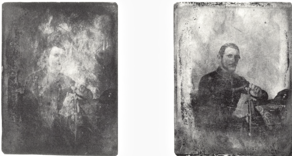
Figure 2. Daguerrotype photograph before (a) and after (b) cleaning in a glow discharge by 'physical' and 'chemical' sputtering (courtesy of W. Poschenrieder).
